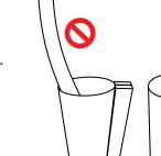
Never pull on top edge with pump hose as weld can unpeel.
