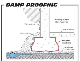
Leave screed boards & stakes in position. Pull Fastfoot® off screeds and tape two edges together on top of footing with 2" sheathing tape. Form and pour wall. After stripping (if required) run 12" width of peel & stick membrane along top of footing (covering staple holes in Fastfoot®) and up side of wall. Lap bottom edge of wall membrane over vertical peel & stick. On the inside, tape underslab membrane to interior Fastfoot®.
