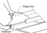
Place one hand on correct 'Fastfoot width line' on ground and bring fabric edge spugly over
