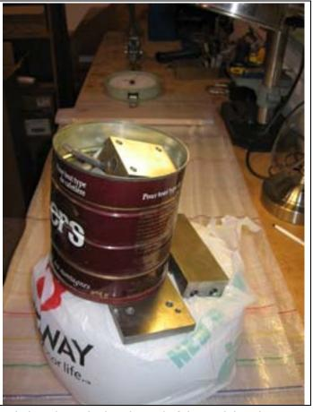
One end of the fabric was wrapped around a 1"x2", stapled, and attached to the end of the work bench. A second piece of fabric was wrapped around a 1"x4" and attached to a spring scale and pulling mechanism.
