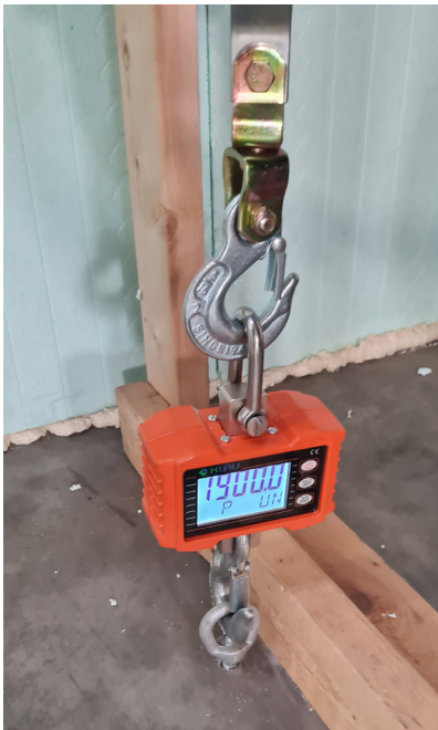
Figure 9: View of scale connected to slab and strap puller. Vertical load test.
