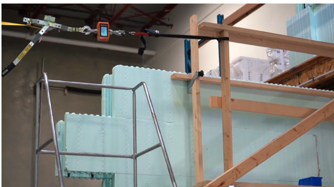
Figure 11: Application of longitudinal load at end post.
